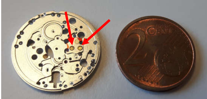
Figure 13. Uneven component with a 1 mm crater (marked by red arrow) beside a European 2-Cent-Stück (diameter: 18.75 mm) for size comparison
