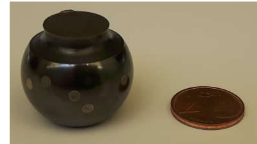
Figure 8. Curved nitrocarburized sample with analysis spots beside a European 2-cent coin (18.75 mm diameter) for size comparison
