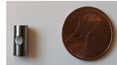
Figure 10. Cylindrical sample with crater
