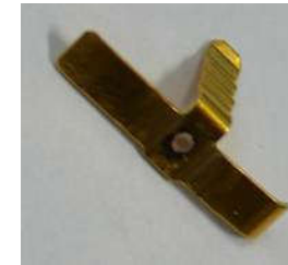
Figure 12. Electrical contact with crater
