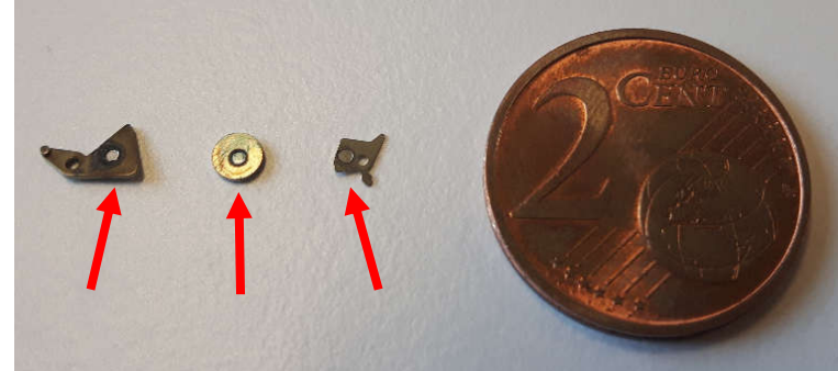
Figure 14. Tiny components with 1 mm craters (marked by red arrow) beside a European 2-Cent-Stück (diameter: 18.75 mm) for size comparison
