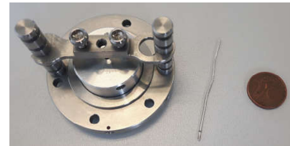
Figure 18. Aluminum wire beside the Universal Sample Unit for wires and a 2-cent-coin for a size comparison
